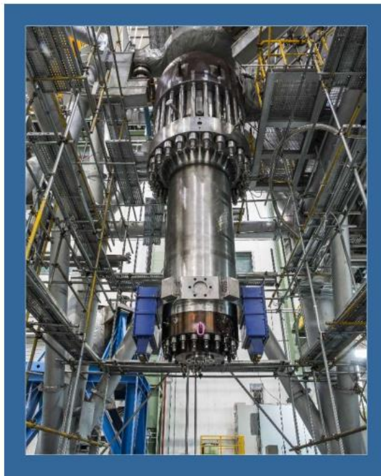
Displayed above is a KSB reactor coolant pump. Source: KSB SE & Co. KGaA, as of March 2023.
